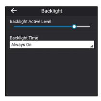
Backlight is configurable via web user interface at the path **Settings**->**Preference**.
